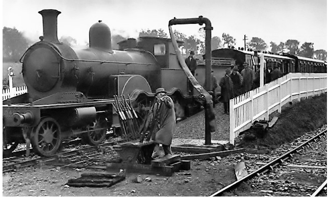
Southern Railway Ex-LSWR “460” Class 4-4-0 on the North Devon and Cornwall Junction Light Railway at Hatherleigh on 28th July 1925 Colonel Stephens Museum
