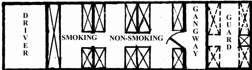
Albyn's suggested seating arrangement for the Pickering railcar
