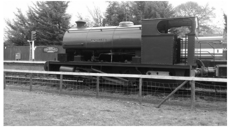
Peckett 0-4-0ST "Achilles" that will run some steam services on the EKR this year
