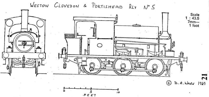
THIS DRAWING IS NOT 100% ACCURATE, BEING BASED ON THE MANNING WARDLE 'M' CLASS LOCO WHICH NOS CLOSELY RECENTLES OF HAS THAT ALERATIONS MADE IN ACCORDANCE TO PHOTOS CURRENTLY AVAILABLE OF NOS
